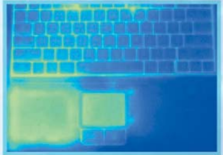
Thermal Image of a Laptop PC Left Palm Rest and Touchpad with eGraf SpreaderShield Thermal Solution, average palm rest temperature 34.5 °C.
