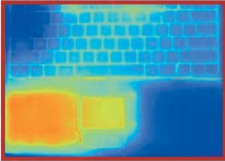
Thermal Image of a Laptop PC Left Palm Rest and Touchpad, average palm rest temperature 42.0 °C.
