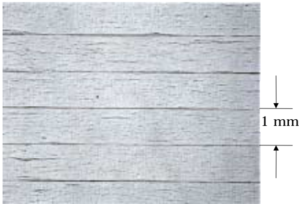
Figure 2 - Polished Cross-Section Through Graphite Laminate.
