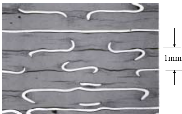
Figure 3 - Polished Cross-Section of Graphite/Copper Laminate.
